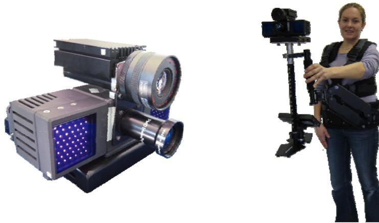
**Figure 1:** 2D-3D-Camera system
