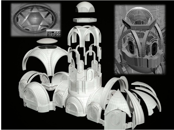
Figure 3. The geometrical complexity of the vault system in an exploded perspective
