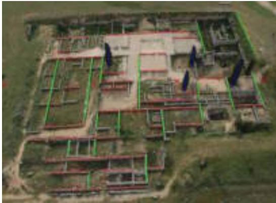
Figure 6. Camera self-calibration supported by oblique image geometry: extraction of vanishing lines and points
