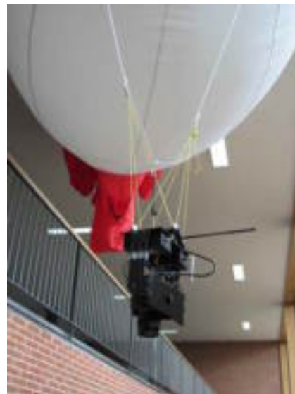
Figure 1. Zeppelin and Picavet system.
