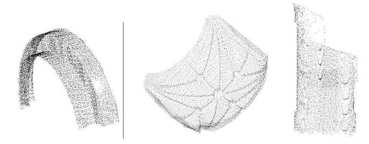
**Figure 6**: Low-resolution models provide a coarse approach to the original surface with the corresponding triangulations which simplifies the detection and suppression of outliers for shape estimation.
