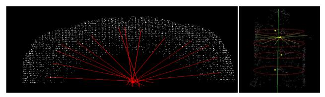
**Figure 7**: 1) Normal vectors of triangles for a low-resolution sample of a spherical vault give the concentration of their intersections around a point at the centre of a sphere. 2) Two consecutive slices of a cylindrical element from a low-resolution sample of a column determine a slab. The intersection of normal vectors gives points which would lie ideally on the cylinder axis. Meaningful deviations of the line connecting them are reported
