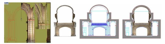
Figure 2: Polylines for arcs and profiles are manually drawn over CAD files arising from points clouds.
