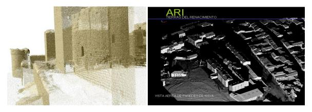
**Figure 3**: Lack of verticality and torsional buckling of walls is one of the most common defects which can be evaluated by computing the difference with respect to ideal geometric primitives.
