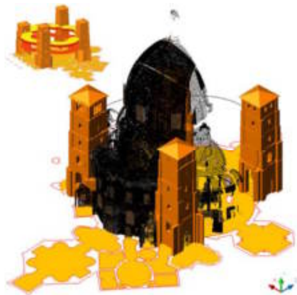
Figure 7. At the top left, identification layout of the towers for the ancient connection route (theoretical) in yellow and the current route in red, at the level of the extrados of the gallery. At the bottom, a 3D view of the nucleus of the Basilica in relation to the towers
