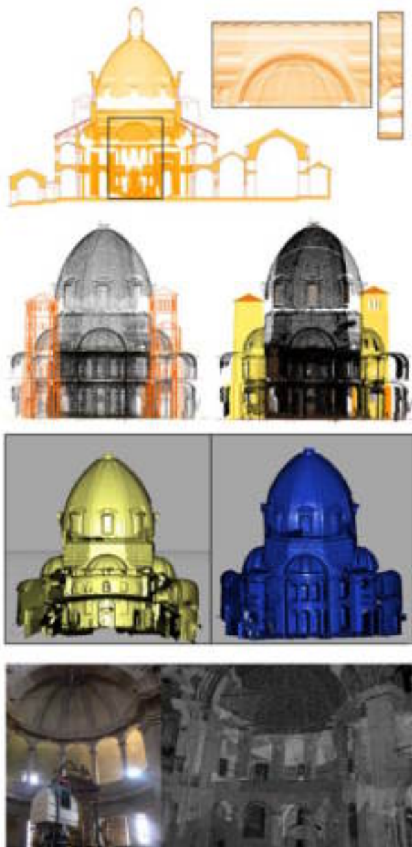
Figure 8. A preliminary raw elaboration of the model and the two ambulatories of the clover-leaf. An additional development seems to need to pass through generation of surfaces (for example, columns and vaulted surfaces) integrated by border line, rather than staying on lines of discontinuity
