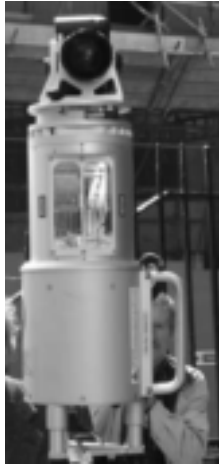
Figure 1. RIEGL LMS-Z420i with a Nikon D100 camera used for the survey.
