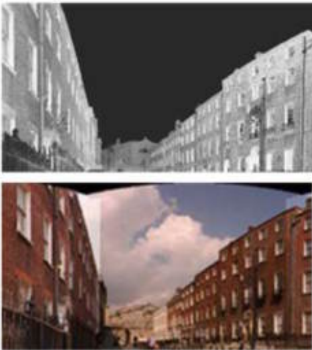
Figure 2. Above the point cloud with the associated image below it, the laser scan collects a large range of data representing three-dimensional co-ordinates, called “point cloud data”. The combination of digital photography and laser scanning enhances the point cloud data, defining edges and texture.
