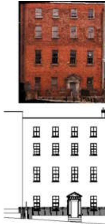
Figure 7. CAD plot from laser scan
