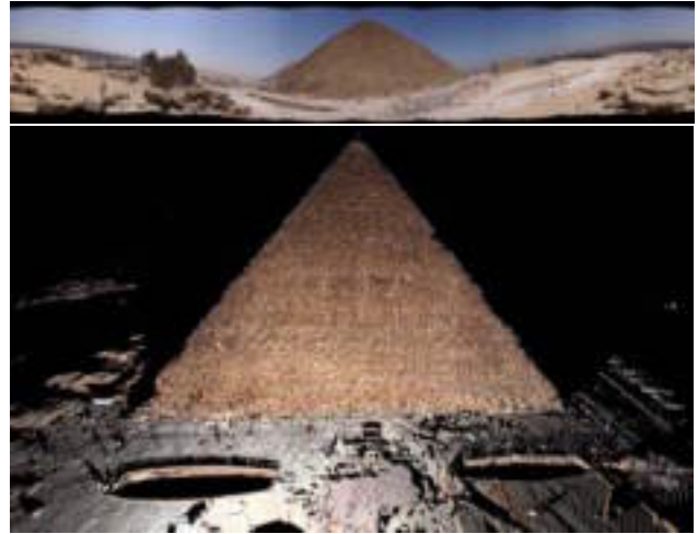
Fig. 5: One single scan from the east front of the Cheops Pyramid visualised in RiSCAN PRO 1.1.2 \beta as coloured point cloud in 2D view (above) and 3D view (below)
