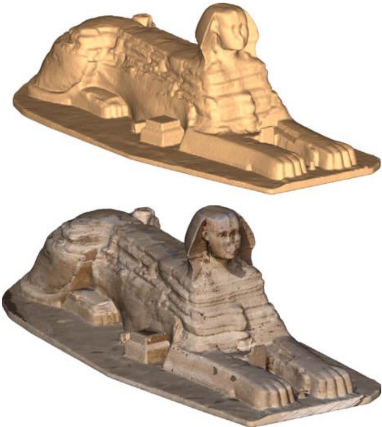
Fig. 7: Triangulated point cloud of the Sphinx combined from 7 scanner positions: 6 from the ground and one from the Cheops Pyramid, triangulated and textured in RiSCAN PRO 1.1.2 \beta
