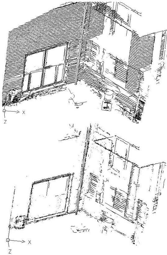
Figure 4. Extracted edges exported in CAD, before (top) and after the geometric edge filtering (bottom)
