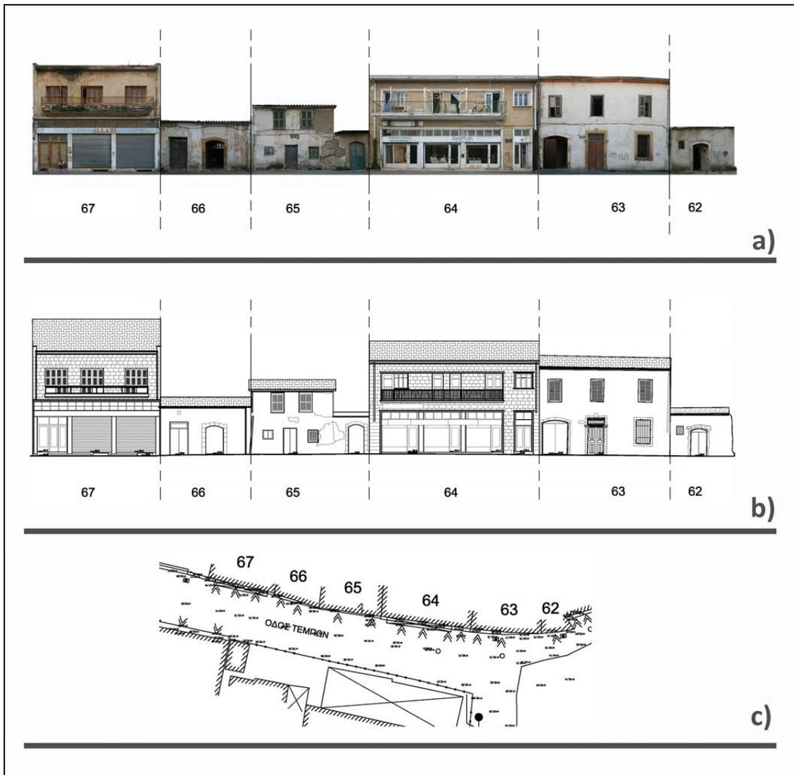
**Figure 8:** Georeferenced Façade series along a street part a) Rectified images b) Architectural Drawings c) Survey Map.
