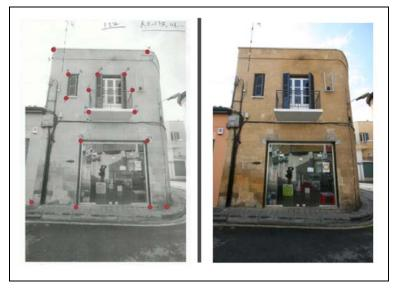
Figure 4: Sample control point sketch and acquired image.
