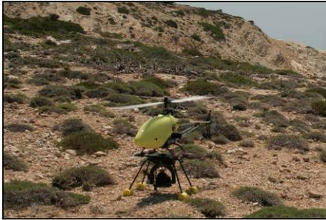
Figure 6: The UAV-helicopter used for the image acquisition.
