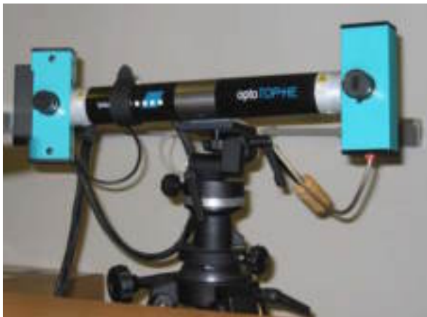
Figure 1. optoTOP-HE-600 fringe projection measurement system
