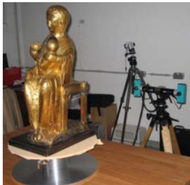
Figure 2. The Golden Madonna positioned on a turning table and the measuring system in the restoration workshop of the Essen cathedral
