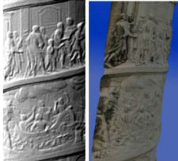
Figure 2: Left: Section (3×6m 2 ) of the surface model with 2cm resolution derived from the Riegl data. Right: a rotated view of the respective section in the 3D-photomodel.
