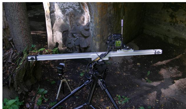
Figure 1. Optical Correlation Scanner
