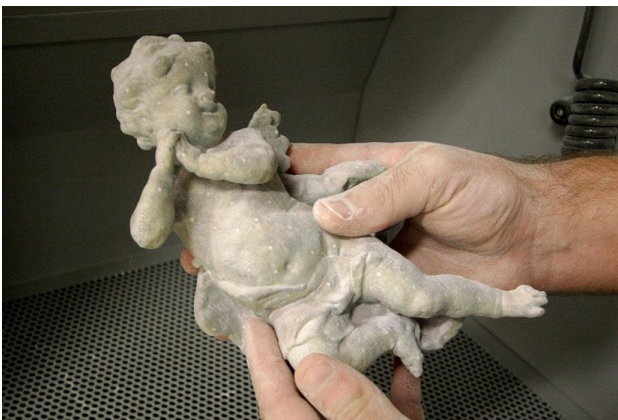
Figure 11. Real 3D colour model from rapid prototyping machine (ZPrinter 450). Stone sculpture of the angel from Mary's pillar by Matyáš Bernard Braun dated in the Baroque era.
