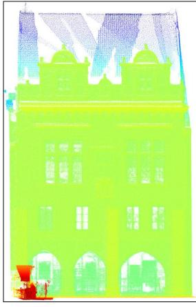
**Figure 4:** Ortoimage in a hypsometry model. Intensity represents the Z-coordinate value.
