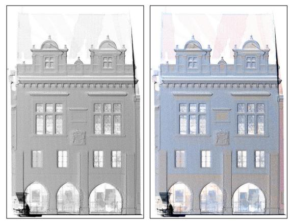
**Figure 3:** a – Density ortoimage. Intensity represents the point density in pixels. b – The same ortoimage as a, including "false" colours.
