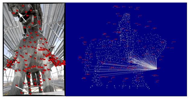
Figure 2: The white arrows on the left image point to the two tie points. Their distance is aproximately 7 m. Right image shows all the rays of this camera station.
