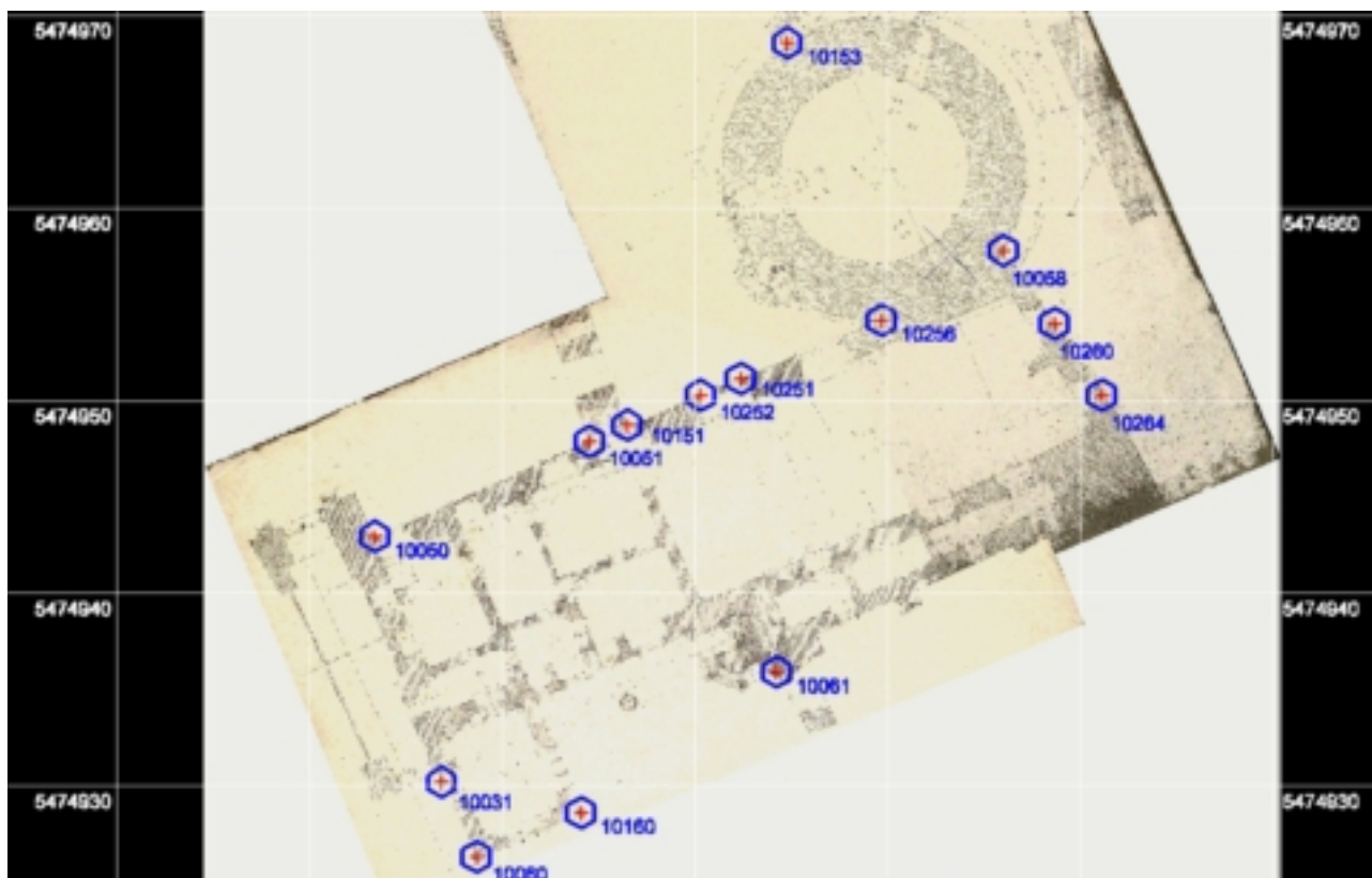
Figure 5: Rectification and combination of two plans presenting the horizontal structure of the “Gläserner Saalbau” made by T. Peschel, Karlsruhe 2003.
