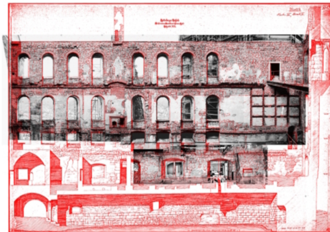
Figure 6: Overlaying of the Koch/Seitz plan and the rectified image (north wall).
