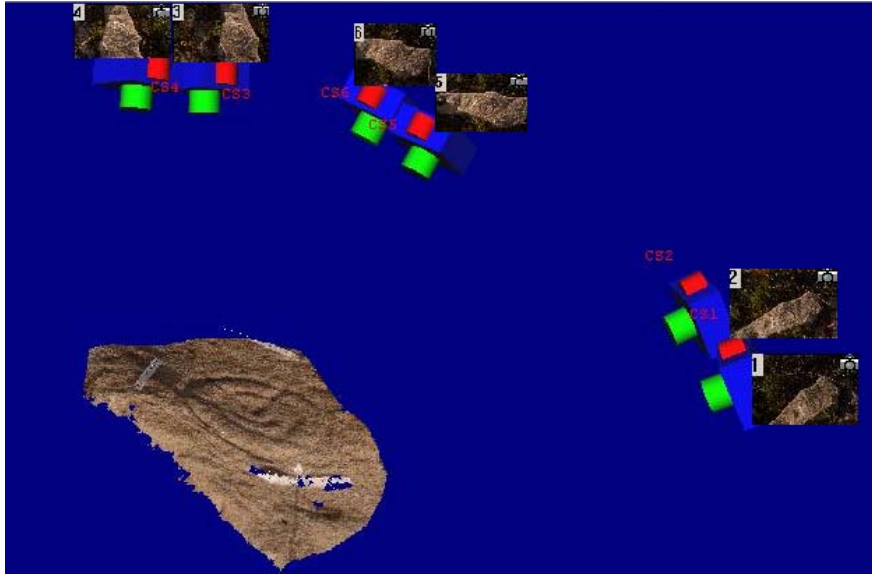
Figure 1: Camera network during image acquisition. Three main camera positions with maximum convergence angles around 90 degrees.
