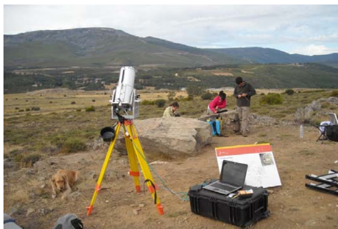
Figure 3: Data acquisition with RIEGL Z-390i scanner from one of the scanner position.
