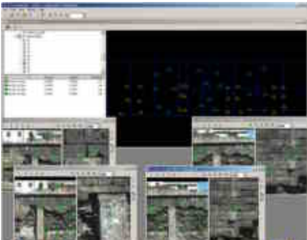
Figure 8. The SV Triangulation module of the Stereo View software produced by Menci Software of Arezzo
