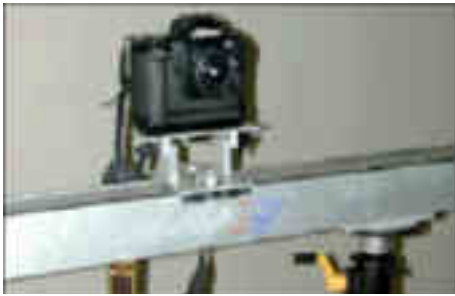
Figure 4. Calibrated aluminium bar on which the digital photcamera used for the photogrammetric survey is positioned
