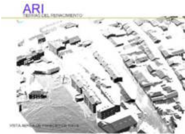
Figure 6: Partial view of the 3D model of Paredes de Nava (Palencia) taken with ILRIS 3D for coarse urban surveying
