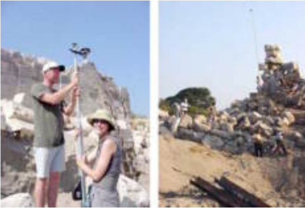
Fig. 2.1 Gaining high resolution digital close range aerial stereoviews of antique sites in PATARA (Turkey) with a single lens staff Canon Powershot camera (approx. 10 m altitude)
