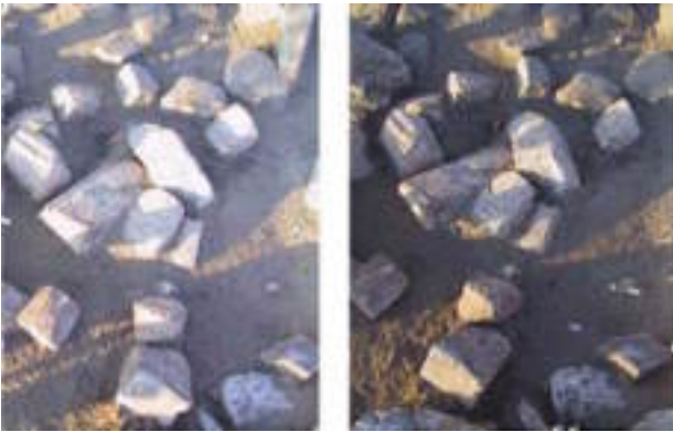
Fig. 2.2 Sample of a high resolution digital close range aerial stereoview of remains of the antique houses of parliament in PATARA(Turkey) (Canon Powershot single lens staff camera, approx. 10 m altitude)
