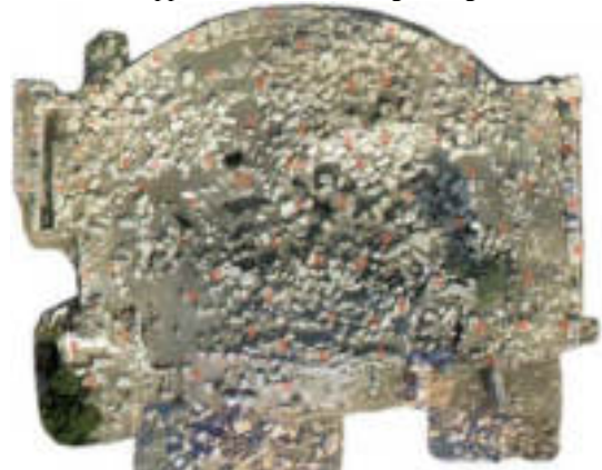
Figure 2.5 Rectified and mosaiced aerial balloon views of the antique houses of Parliament at the archaeological site of PATARA (Turkey), as carried out by B. Luebbehusen
