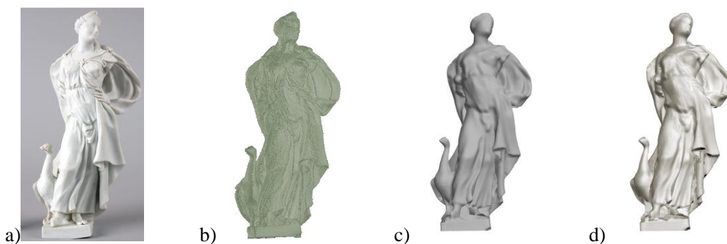
Figure 8. Biscuit: a) photo [20]; b) cloud of points; c) triangle mesh; d) triangle mesh with texture.
