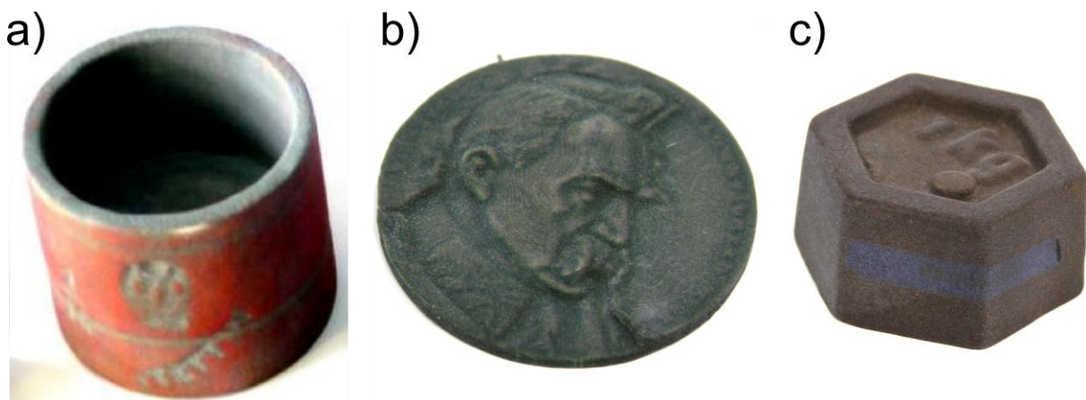
Figure 7 Printed copies of the measured objects: a) volume reference cup; b) occasional medal; c) weight reference.
