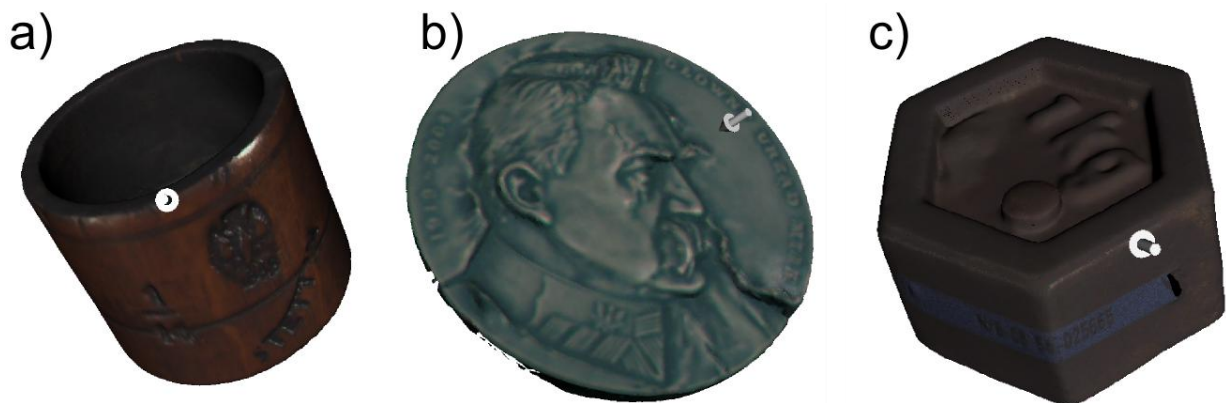
Figure 6 Models of measured objects: a) volume reference cup; b) occasional medal; c) weight reference.
