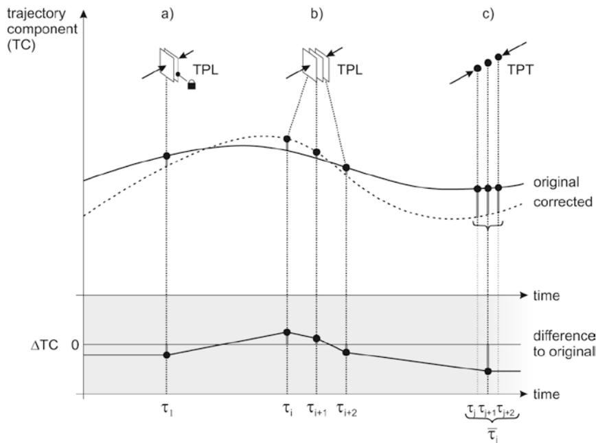
**Figure 4:** Examples of applied trajectory corrections at specific time-stamps (vertices) based on tie observations in the point cloud.
