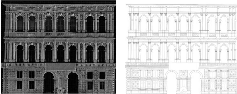
**Figure 6:** (left) Orthoscan with gray-scale coded reflectance (*RIEGL RiPROCESS/RiSCAN PRO*) and (right) 2D CAD Drawing (*EKG*) of "Casa Pesaro".
