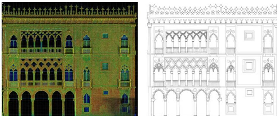
**Figure 5:** (left) Orthoscan with color-coded reflectance (RIEGL RiPROCESS/RiSCAN PRO) and (right) 2D CAD Drawing (EKG) of “Casa d’Oro”.
