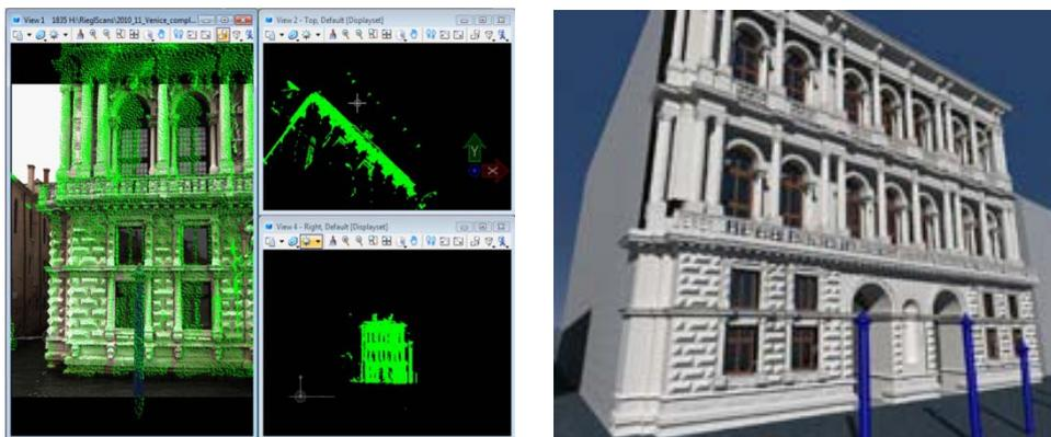
**Figure 7:** (left) 3D Monoplotting and 3D CAD drawing (*Phocad/Phidias*) of "Casa Pesaro".
