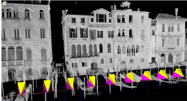
**Figure 2:** Illustration of the camera positions and fields of view at the moment of their synchronous trigger. Yellow and pink cones represent the fields of view of camera 1 and 2, respectively. The thin red line describes the trajectory. Scan data is displayed colored with the gray-scaled relative reflectance.
