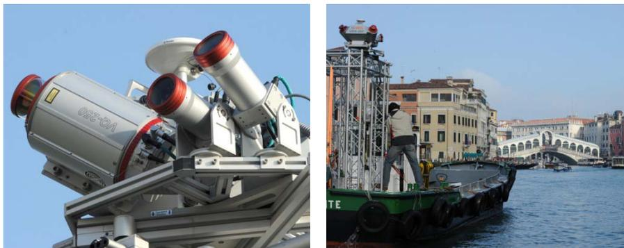
**Figure 3:** (left) *RIEGL* VMX-250 mobile laser scanning system with the modular camera system and (right) mounting of the system on the workboat “Sante” during scanning.
