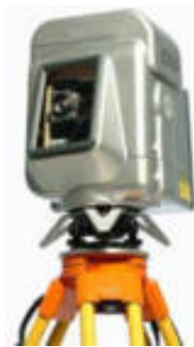
Figure 2. GS200 laser scanner ( www.mensi.com )
