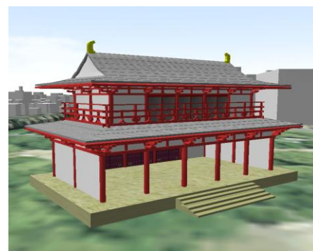
Figure 15 The parameters (the slope of roofs, the standard interval of pillars and so on) are changed
