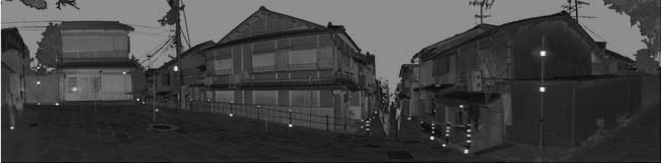
Figure 4: Two-dimensional image of TLS data measured in front of Hohkanji-temple, Higashiyama-ku, Kyoto.
