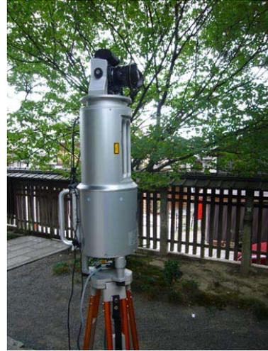
Figure 3: Terrestrial laser scanner used for the measurement (LMS-Z360i, produced by Riegl)
