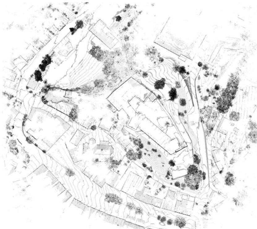
**Figure 3:** The contour map of the area generated from point cloud
