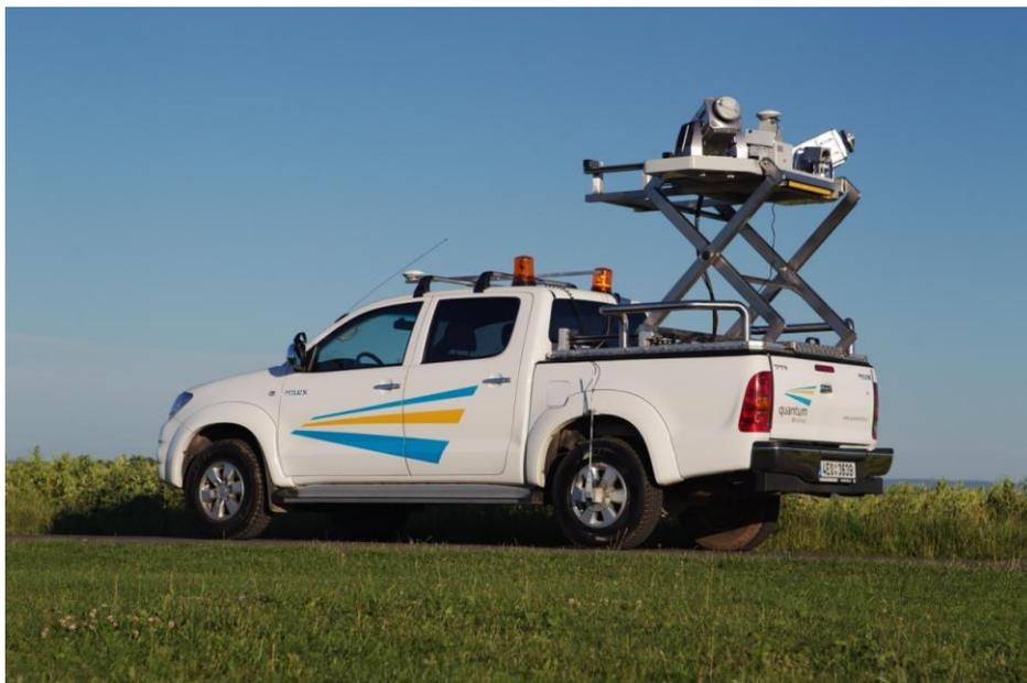
**Figure 2:** Lynx Mobile Mapper platform placed on a car body
