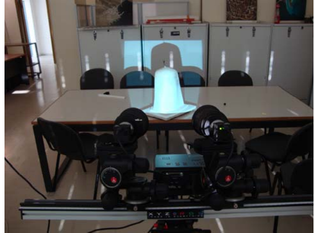
Figure 8. XYZRGB™ structured light scanner setup for the acquisition of data for the plaster model
