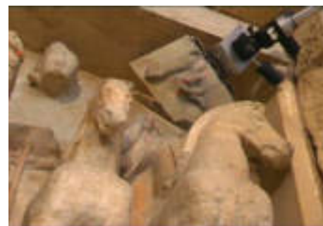
Figure 4. Practical considerations when using a 3D scanner: mirror used to reach hidden 3D surfaces.
