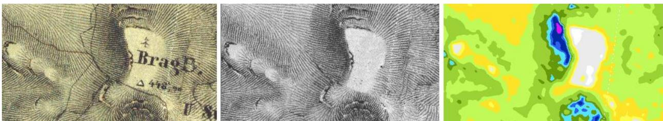
**Figure 5:** Original map drawing (on the left), map drawing after removing the planimetric objects and descriptions (in the middle), areas of constant slope (on the right).
