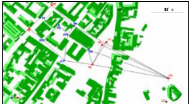
Figure 11. Topographic net: in blue vertexes measured by EDM only, in red measured also by fast-static DGPS.
