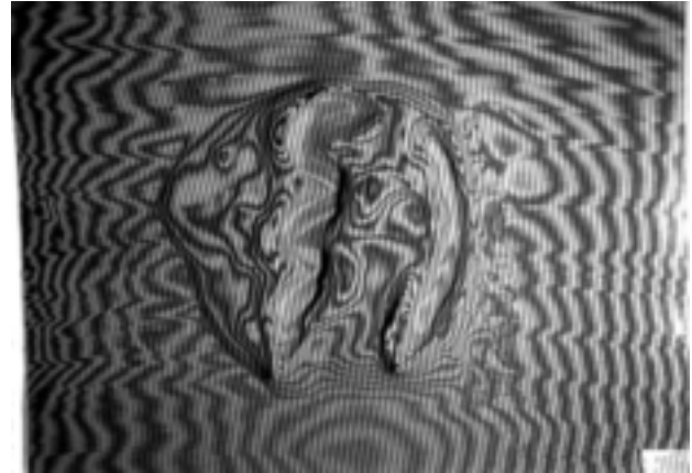
Figure 18. Wet Mud Figure Model with Moiré Screen
