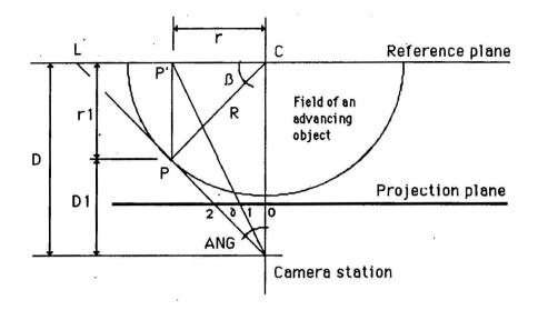
Fig. 1: Deformation in cylindrical or spherical objects.
