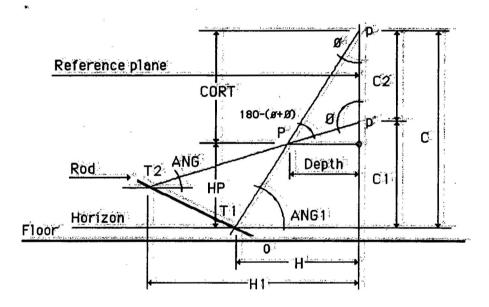
Fig. 2: Stereoscopic exposure with the camera tilted on one plane, perpendicular on the other.
